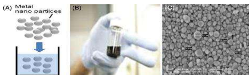
Figure (A) Basic concept to explain metal ink preparation concept, (B) Silver NP ink in a small vial, and (C) HR-SEM of particle after evaporation of the solvent.
