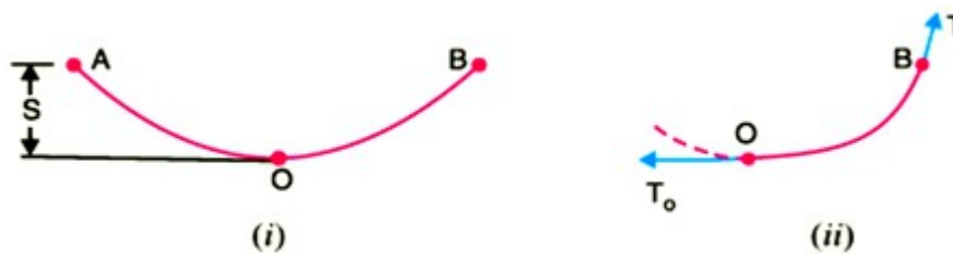
Figure 3.1 Sag in Overhead lines
